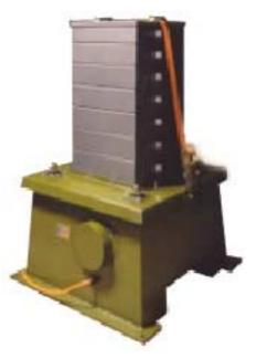
netic vibrator integrated into the oscillating table to assure optimum screening efficiency.
