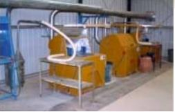
LM5 mills installed at a commercial assay laboratory in Kalgoorlie, Western Australia. Note this customers preference to install their own (white coloured) flexible vacuum hoses for final bowl cleaning and their introduction of a coarse dust trap between the mills and their dust extraction ducting
