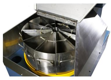
ALL PARTS IN DIRECT CONTACT WITH THE SAMPLE ARE OF STAINLESS STEEL CONSTRUCTION (except on models 130 & 200 which are mild steel)
