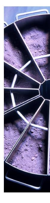
Buckets are fitted with handles for easy removal. Turntable can be free -wheeled by hand to bring each bucket to front of unit
