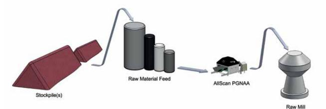
In both applications the data from the **AllScan** is seamlessly transferred to the plant control system and is typically interfaced to 3rd party QC optimization software to improve quarry operations, stockpiling and raw mix proportioning.
