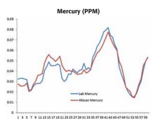
Measurement of trace elements, e.g. Mercury, Selenium, Arsenic, etc. at PPM levels.
