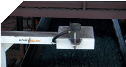
**MoistScan®** MA-500HDI measuring moisture content of iron ore pellets at a shipping port. The analyser is used to calculate the total dry tonnage as the product is loaded onto the ship.
