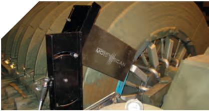
**MoistScan®** MA-600 installed on a vertical disk filter at a copper processing plant. The analyser measures the moisture in filter cake. Data from the **MoistScan®** controls the vacuum pressure of the filter plates to produce a filter cake within a tight moisture specification of 7-8%.
