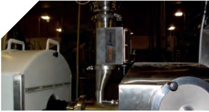
**MoistScan®** MA-700 analyser installed on the in-feed to a hydrator at a snack foods factory. The analyser measures the moisture in a mixture of polenta and rice. Data from the **MoistScan®** directly controls moisture addition to the hydrator to ensure the product meets quality specification.
