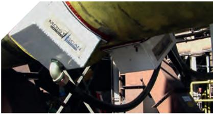
**MoistScan®** MA-600 installed on a large screwfeeder conveying woodchips to a dryer at a wood char plant. Data from the **MoistScan®** is used to control the dryer such that the woodchip exiting the dryer is between 5-12% moisture.
