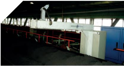
**MoistScan®** MA-500 installed on the coal receival belt of a power plant. The MA-500 is used in conjunction with an online elemental analyser to determine the total dry ash percentage and sulphur content of the received coal.
