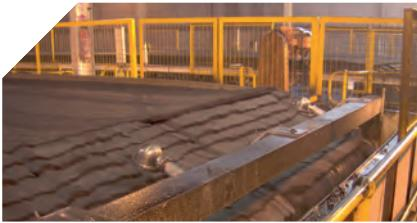
**MoistScan®** MA-600 installed on a horizontal belt filter at a coal wash plant. The MA-600 has 3 sets of antennae across the belt. The analyser calculates average moisture across the belt which is used to control belt speed and flocculant addition.
