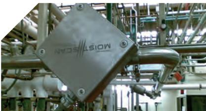
**MoistScan®** MA-500HD installed on the plant feed conveyor belt at a nickel ore refinery. Data from the **MoistScan®** is used to control the residence time of the ore in a rotary dryer.
