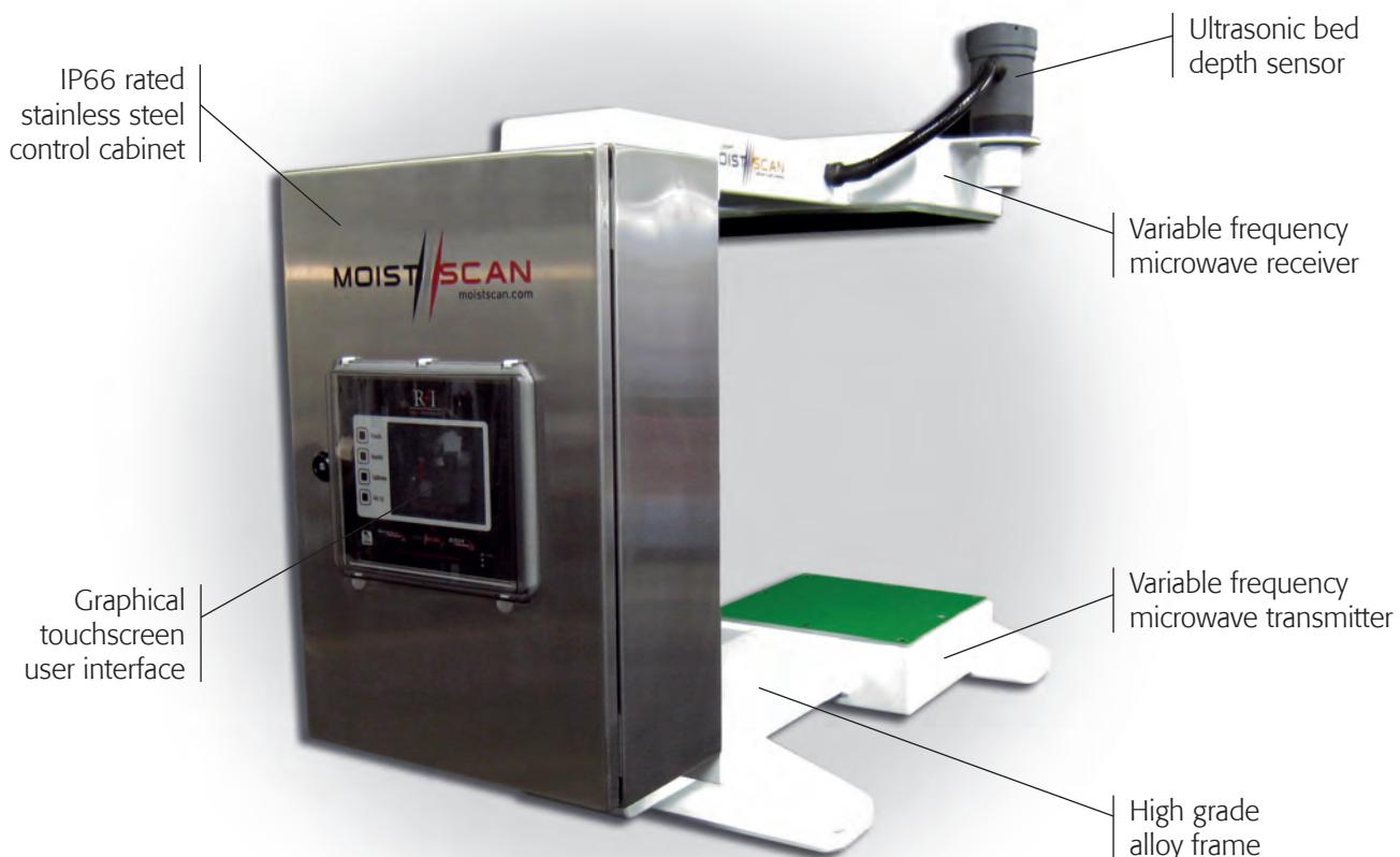
Our patented **MoistScan®** dual measurement multi-frequency microwave generator measures attenuation and phase shift of the microwave signal at discrete pre-defined frequencies.
